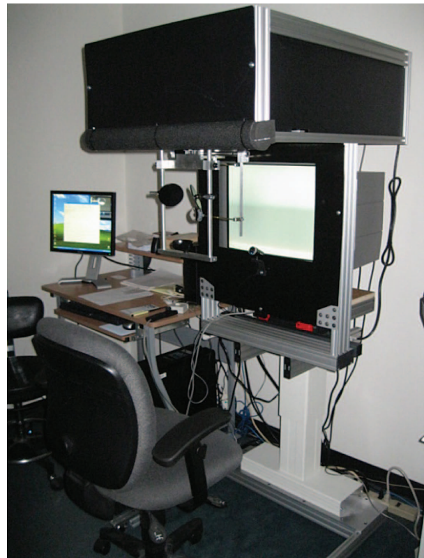
Figure 3. Customized testing station of contrast sensitivity perimetry.
